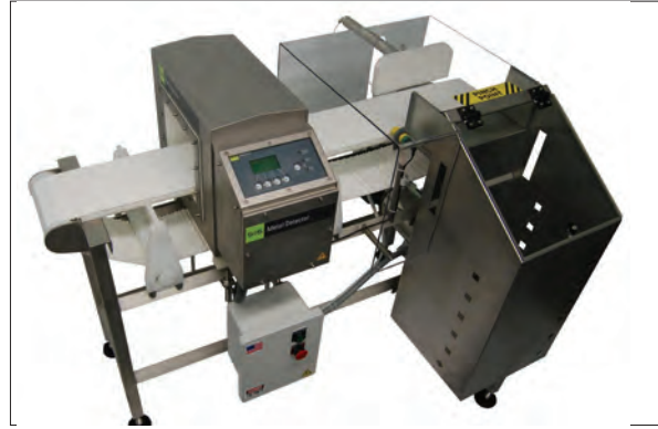
Optional reject bin for safe storage until QA can identify contaminants
